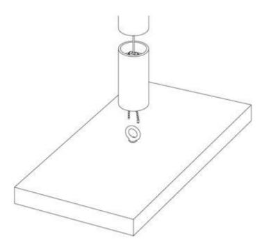
Pass a ball chain through the bottom ring of a rain chain and connect to an anchor.
