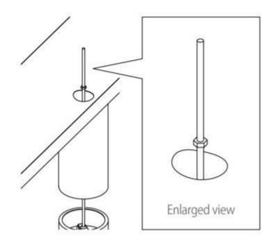
Put a long bolt through the centre hole in a bracket and screw a second hexagon nut tightly.
