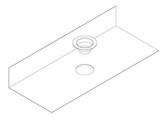
After attaching a designated long bolt on the top of a rain chain, screw a hexagon nut onto a long bolt, then pull up through a stainless-steel gutter outlet.
