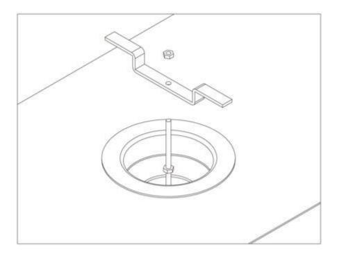
Screw a wing nut tightly on top of a hexagon nut.
